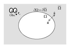
$$\phi(\mathbf{r}_{o}) = \iiint_{\overline{\Omega}} \frac{\rho(\mathbf{r}_{s})}{\mathcal{E}} G(\mathbf{r}_{o}; \mathbf{r}_{s}) dv_{s} + \oiint_{\partial \overline{\Omega}} \left\{ \underbrace{G(\mathbf{r}_{o}; \mathbf{r}_{s}) \frac{\partial \phi(\mathbf{r}_{s})}{\partial n'}}_{\mathbf{e} \mathbf{n} - \mathbf{p} \mathbf{n}} - \phi(\mathbf{r}_{s}) \frac{\partial G(\mathbf{r}_{o}; \mathbf{r}_{s})}{\partial n'} \right\} dS_{s}$$
